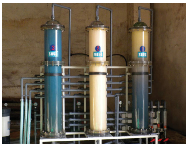
Figure 7. A set of three packed columns for Ni hydrometallurgical extraction of low-grade nickeliferous laterites.
